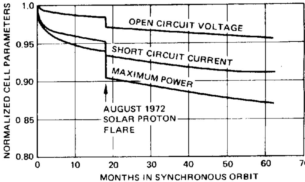
Figure 15.1: Degradation of the solar cell array on a spacecraft with time due to damage by energetic particles [Goldhammer et al., 1976]. The step function decrease was due to the protons from one large solar flare.
