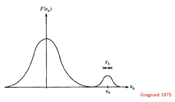
Langmuir wave excitation/damping is prop to gradient of distribution in velocity space.
