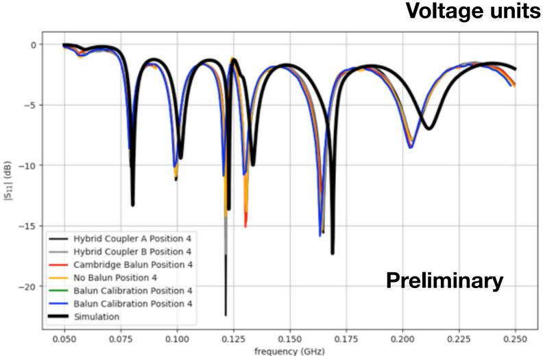
Sinuous Feed Growth-Rate = 0.8 100 Ohm termination
