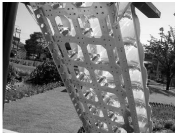
Figure 7: CPV for “Breeding Plants” that collects direct beam and provides diffused sunlight to the underneath plant.
